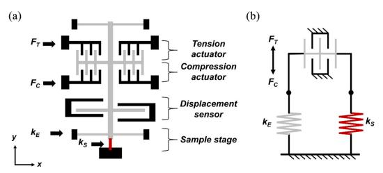
Fig. 1 Schematics of the structure (a) and lumped mechanical model (b) of the tension-compression MEMS device.
