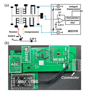
Fig. 3 (a) The schematic of the test system setup based on the MEMS device. (b) The PCB contains the wire-bonded MEMS device and capacitive readout circuit.
