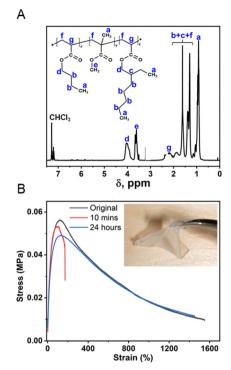
Fig. 3 (A) <sup>1</sup>H-NMR spectrum of the matrix polymer with characteristic chemical shift peaks marked on the chemical structure. (B) Tensile results of the cut matrix polymer that self-healed for 10 min and 24 h in comparison to the original uncut material.
