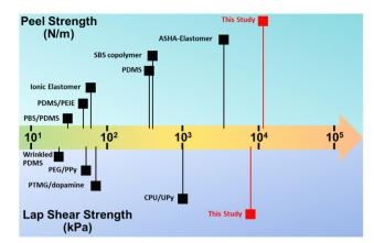
Fig. 6 Summary of adhesion performance of currently reported advanced ductile adhesive elastomers, including the reported chemistries: ASHA-elastomer, 25 SBS copolymer, 39 PDMS, 21 ionic elastomer, 48 PDMS/ PEIE, 49 PBS/PDMS, 64 CPU/UPy, 47 PTMG/dopamine, 27 PEG/PPy, 46 and wrinkled PDMS.50
