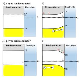
Fig. 1 Energy diagrams for n-type and p-type semiconductor electrodes immersed in an electrolyte with electrochemical potential ( $E_{FC}$ ) at nonequilibrium (a) and (c) and in equilibrium (b) and (d) with the Fermi level of the semiconductor  $(E_{\scriptscriptstyle E})$ .
