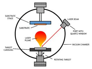
Fig. 7 Scheme of pulsed laser deposition equipment.
