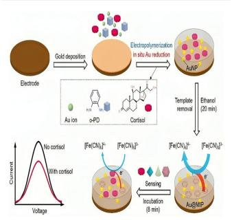
Fabrication process and sensing mechanism of a cortisol sensor on gold doped MIP layer. Adapted and reprinted with permissions 135 Copyright (2015), with permission from Elsevier.
