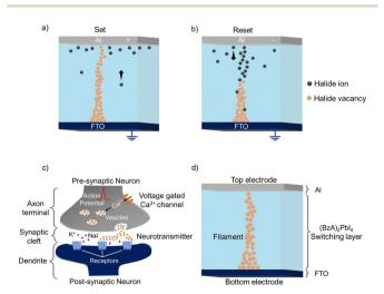
Fig. 4 Resistive switching mechanism in layered hybrid perovskites. Schematic of (a) set (LRS) and (b) reset (HRS) switching governed by ion migration. Illustration of a (c) biological snapse and (d) (BzA)<sub>2</sub>PbI<sub>4</sub>-based artificial synapse mimicking the biological function.
