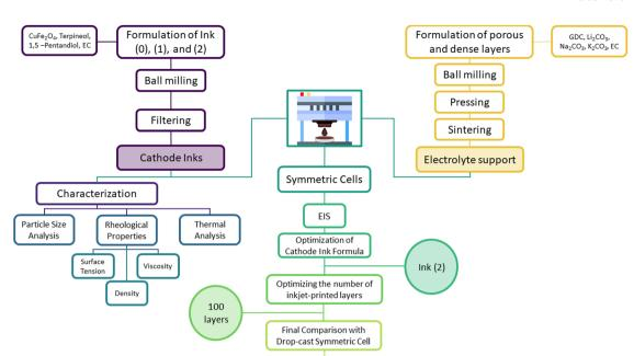
Experimental steps of fabrication, characterization, and optimization for an inkjet-printed CuFe<sub>2</sub>O<sub>4</sub> symmetric cell.
