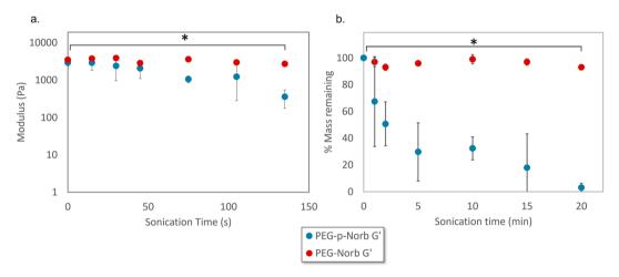
Fig. 3 (a) Change in storage modulus and (b) mass loss of hydrogels when sonication is performed on a hydrogel system (power output of 7 W, 20 Hz, in 10 mL of DI water on ice). The phthalaldehyde containing system displayed a significant decrease in both storage modulus and mass with increased sonication time. Error bars represent mean + one standard deviation, n = 3. p-Values were calculated with Welch's t-test. \* p < 0.05.
