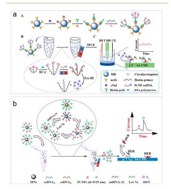
Fig. 1 (a) Magnetic RCA-assisted immunosensor for cTnI detection based on impact electrochemistry. Reproduced with permission from ref. 74. Copyright American Chemical Society, 2022. (b) Schematic of the size-resolved single entity collision biosensing for the quantification of microRNA in a single run using 5 nm and 15 nm PtNPs as electrochemical probes. Reproduced with permission from ref. 76. Copyright American Chemical Society, 2021.
