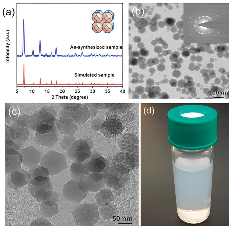
**Fig. 3** (a) X-Ray diffraction patterns of ZIF-8 crystals. (b and c) Transmission electron microscope (TEM) images of ZIF-8 crystals. (d) Suspension of ZIF-8 crystals in methanol. Reproduced from ref. 14 with permission from the Royal Society of Chemistry, copyright 2017.
