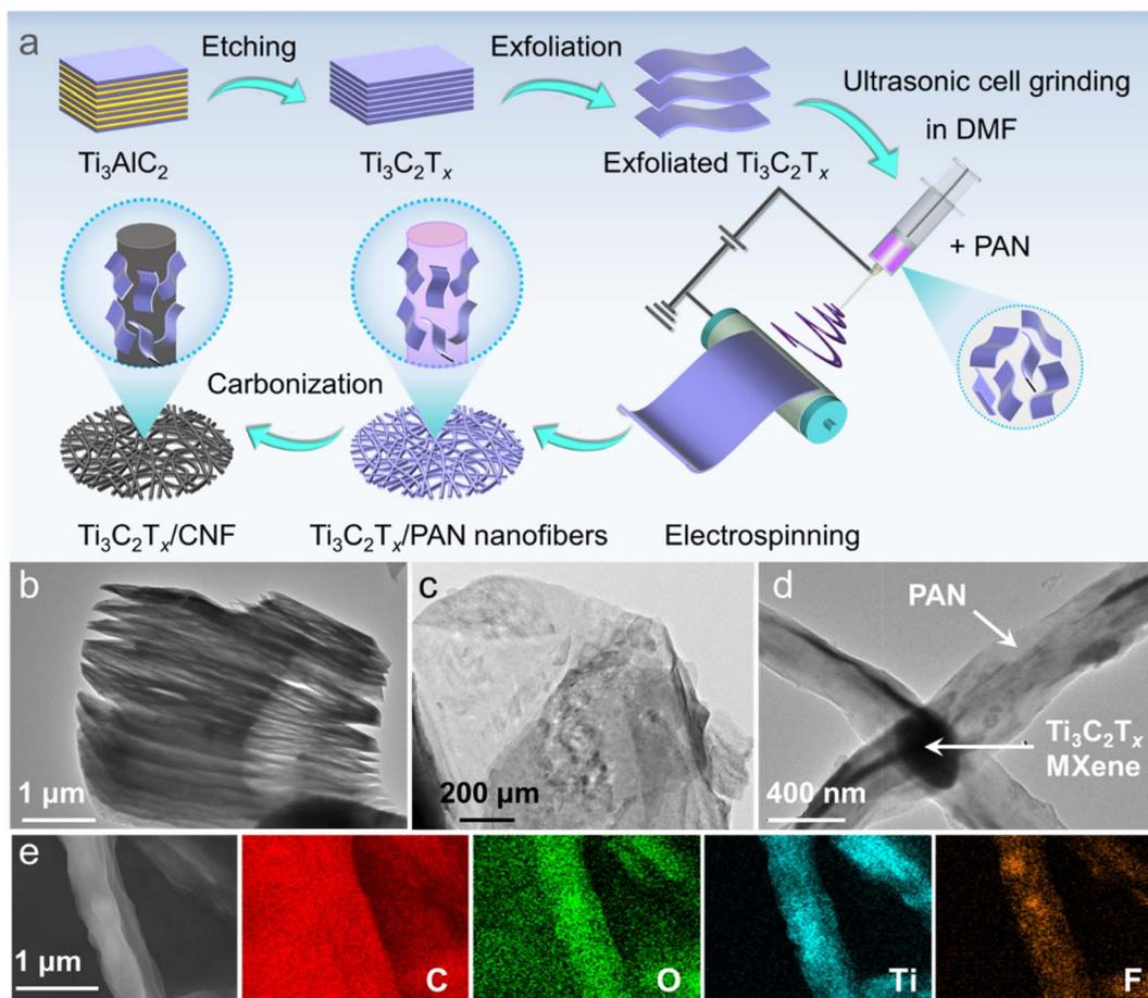
Fig. 1 (a)  $\text{Ti}_3\text{C}_2\text{T}_x/\text{CNF}$  fabrication (schematic). TEM images of etched  $\text{Ti}_3\text{C}_2\text{T}_x$  (b), exfoliated  $\text{Ti}_3\text{C}_2\text{T}_x$  (c), and  $\text{Ti}_3\text{C}_2\text{T}_x/\text{PAN}$  (d). (e) SEM images of  $\text{Ti}_3\text{C}_2\text{T}_x/\text{PAN}$  and corresponding elemental mappings.
