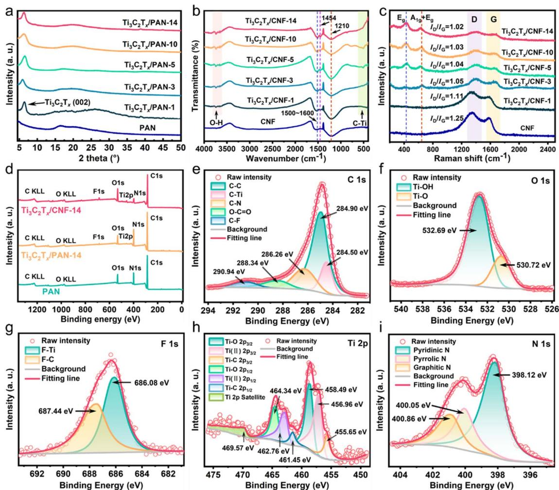
Fig. 3 XRD patterns (a), FTIR data (b), and Raman spectra (c) of samples. (d) XPS surface survey scan spectra of  $\text{Ti}_3\text{C}_2\text{T}_x/\text{CNF-14}$ ,  $\text{Ti}_3\text{C}_2\text{T}_x/\text{PAN-14}$ , and PAN. High-resolution XPS spectra of C 1s (e), O 1s (f), N 1s (g), F 1s (h), and Ti 2p (i) of  $\text{Ti}_3\text{C}_2\text{T}_x/\text{CNF-14}$ .
