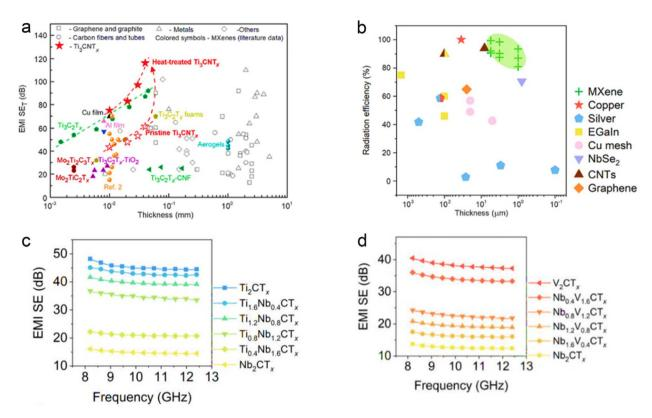
Fig. 19 (a) Comparison of EMI shielding efficiencies of MXenes with carbons and metals. (b) A comparison of radiation efficiency *versus* thickness for MXene with metals, carbons, and others as patch antennas. (c and d) EMI SE of various MXenes with their solid solutions. Reproduced from ref. 337 with permission from [John Wiley and Sons], copyright [2020].
