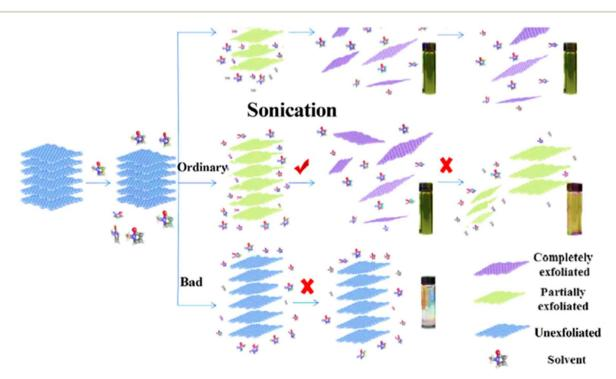
Fig. 9 A schematic illustration of the liquid-phase exfoliation method. 191
