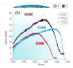
Fig. 17 (a) Calculated elastic constant values for various MXenes. (b) MXene stress-strain curves for Ti<sub>2</sub>C, Ti<sub>3</sub>C<sub>2</sub>, Ti<sub>4</sub>C<sub>3</sub>. Reproduced from ref. 15 with permission from Springer Nature, copyright 2017.
