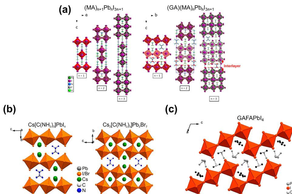
Fig. 6 Crystal structures of (a)  $(MA)_{n+1}Pb_nI_{3n+1}$  and  $(GA)(MA)_nPb_nI_{3n+1}$  (right),  $n = 1, 2$  and 3. Reproduced with permission.<sup>56</sup> Copyright 2017, ACS Publishing Group. (b)  $(GA)(Cs)_nPb_nX_{3n+1}$  ( $n = 1$  and 2;  $X = I$  and Br) Reproduced with permission.<sup>57</sup> Copyright 2017, ACS Publishing Group; (c)  $GAFAPbI_4$ . Reproduced with permission.<sup>34</sup> Copyright 2018, ACS Publishing Group.
