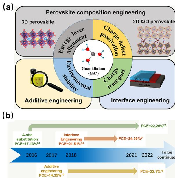
Fig. 1 (a) The schematic diagram of strategies for the GA<sup>+</sup> cation in the PSCs. (b) The development of GA<sup>+</sup>-based PSCs.
