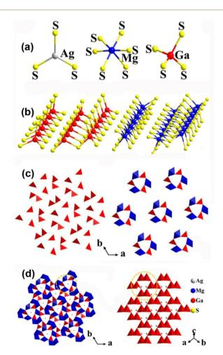
Fig. 11 (a) Coordinated environment of [AgS<sub>3</sub>], [MgS<sub>6</sub>], and [GaS<sub>4</sub>] atoms; (b) 1D [GaS<sub>4</sub>], [Ga<sub>2</sub>S<sub>7</sub>], [MgS<sub>6</sub>], and [Mg<sub>2</sub>S<sub>9</sub>] chains; (c) 1D Ga-S chains and  $[Mg_3Ga_3S_{24}]$  groups viewed along the ab plane; (d) 3D structure of  $AgMg_3Ga_3S_8$  (left) and  $AgGaS_2$  (right) with the  $[Ga_6S_{18}]$  units marked (yellow dashed circle). Copyright 2022 American Chemistry Society.
