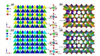
Fig. 8 Crystal structure of  $Li_2MgM^{IV}Se_4$  ( $M^{IV} = Ge$ , Sn): (a and c) 3D diamond-like structures viewed along the c direction; (b and d) 3D channel-like structures viewed along the ab plane.
