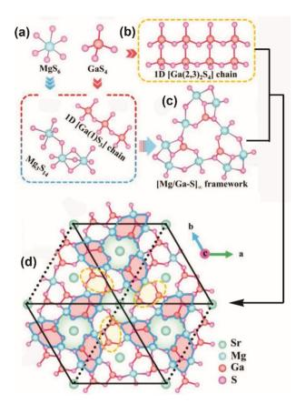
Fig. 6 (a) Coordination environment of [Mg<sub>3</sub>S<sub>14</sub>] trimers and 1D [Ga(1)  $S_3$ ] chain; (b) 1D [Ga(2,3)<sub>2</sub> $S_4$ ] chain; (c) 3D [(Mg/Ga)S]<sub> $\infty$ </sub> framework and (d) crystal structure of SrMg<sub>6</sub>Ga<sub>6</sub>S<sub>16</sub> viewed along the ab plane. Copyright 2022 Wiley.
