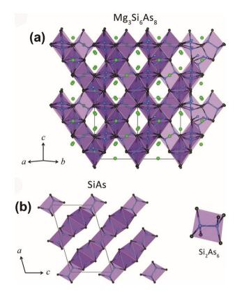
Fig. 3 (a) Crystal structure of the 3D Si-As network in Mg<sub>3</sub>Si<sub>6</sub>As<sub>8</sub> and (b) SiAs with Si<sub>2</sub>@As<sub>6</sub> marked as purple octahedra. Green atom: Mg; blue atom: Si; black atom: As. Copyright 2018 Wiley.
