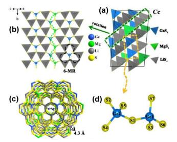
Fig. 4 Crystal structure of Li<sub>4</sub>MgGe<sub>2</sub>S<sub>7</sub>: (a) 3D diamond-like structure; (b) single 2D layered fragment viewed along the [102] direction; (c) honeycomb-like 3D framework with an internal diameter of about 4.3 Å; (d) coordination environment of [Ge<sub>2</sub>S<sub>7</sub>]<sup>6-</sup> dimers. Copyright 2021 Wiley.
