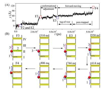
Fig. 7 (A) The time-evolutional trace of the nanoparticle along y-direction at  $D_p = 60$  Å,  $\Delta q = 0.25e$ , and  $\Delta V = 10V_0$ . (B) The snapshots of the nanorobot in the step III-IV (from the state F3 to state F4). In order to clearly discriminate the three legs of the nanorobot in different states, leg1, leg2, and leg3 are highlighted by blue, green, and magenta, respectively.
