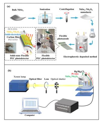
(a) The preparation of the NbSe<sub>2</sub>/Nb<sub>2</sub>O<sub>5</sub>-based PEC photodetector and solid-state PEC photodetector, and (b) photoelectric performance
