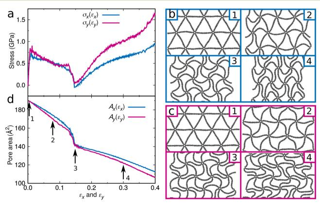
Fig. 2 Graphene foam membrane with an initial pore area of 187 Å<sup>2</sup>: (a) Stress–strain curves for loading in the x- and y-directions. Structure under increasing strain (0.005, 0.075, 0.150, and 0.300) applied in the (b) x- and (c) y-directions. (d) Pore area as a function of the strain applied in the x- and y-directions.
