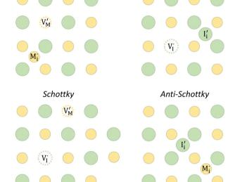
Fig. 1 (a) Perfect crystal of a square metal iodide lattice MI. (b) Electronic disorder involving electronic defects e' and h\*. (c) Different types of ionic disorder involving metal and iodide point defects (interstitials  $I_i'$  and  $M_i^{\bullet}$  and vacancies  $V_I^{\bullet}$  and  $V_M'$ ).
