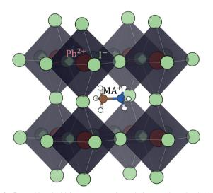
Fig. 4 Perovskite (cubic) structure of methylammonium lead iodide  $(CH_3NH_3PbI_3 \text{ or MAPI})$ . Color code: Pb red, I light-green, C brown, N blue, H white.
