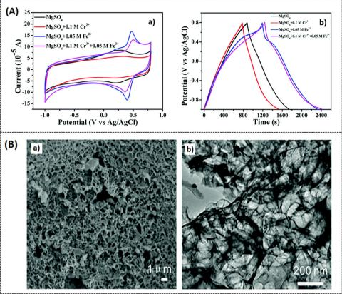
Fig. 15 (A) (a and b) CV response of optimal composite BPGC at different electrolyte medium at a scan rate 5 mV s<sup>-1</sup>, GCD response at 0.5 A g<sup>-1</sup> current density. (B) (a and b) SEM and TEM images of BPGC. Reproduced with permission, 96 Copyright (2022), Royal Society of Chemistry
