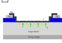
Fig. 2 (a) Schematic of a graphene-on-semiconductor (Si) solar cell. (b) Electron-hole pairs transport across the surface junction. Reproduced from ref. 159, with permission from Elsevier.
