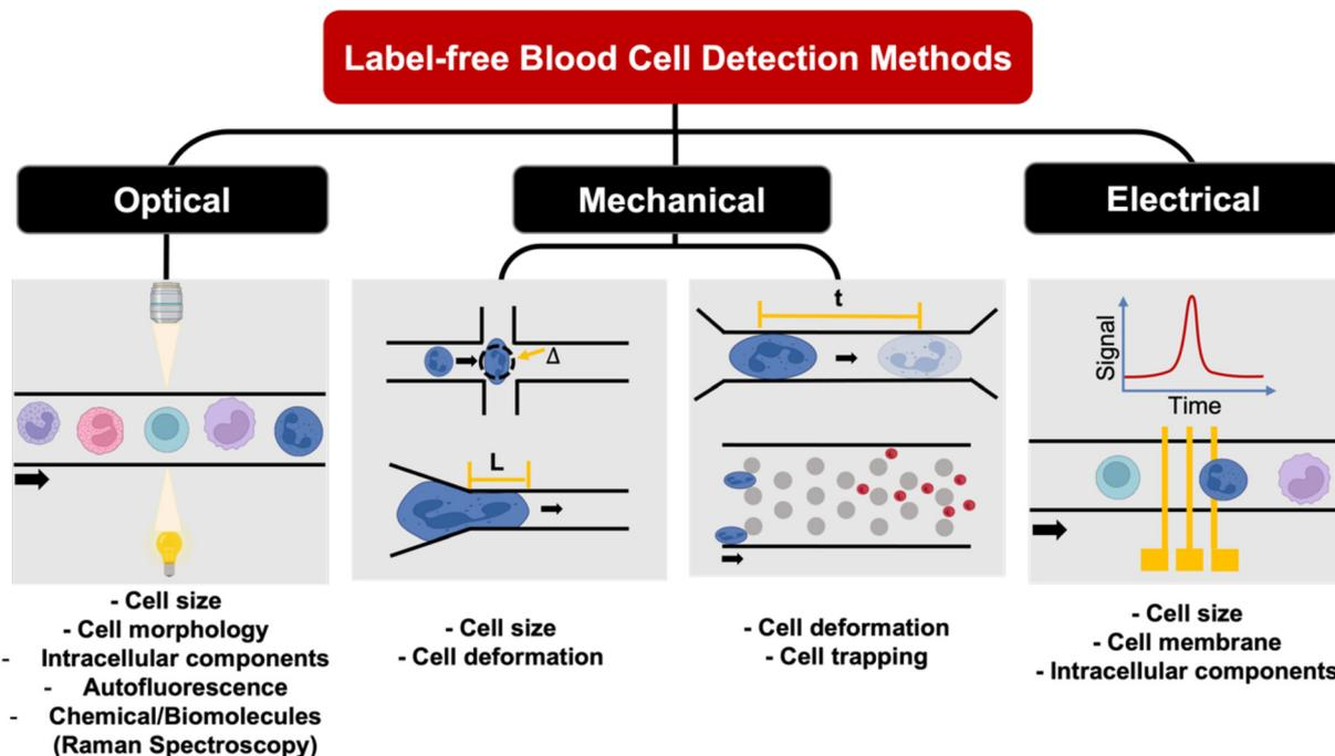
Fig. 8 Overview of microfluidic label-free single cell analysis.
