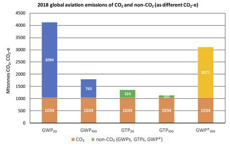
Fig. 20 Emissions from global aviation in 2018, expressed as Mtonnes of  $CO_2$  and apparent emissions of non- $CO_2$ , expressed as various metrics and time horizons. The  $CO_2$  emissions (orange) for 2018 are evidently invariant, whereas the non- $CO_2$ -e emission magnitude varies with metric (blue, GWP; green GTP, yellow GWP\*) and time horizon. Data from Lee *et al.* (2021).
