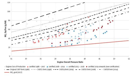
Fig. 2 Engine NO<sub>x</sub> emissions certification data<sup>39</sup> showing the metric as ordinate and the pressure ratio as abscissa. The lines represent the various CAEP standards and goals.
