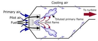
Fig. 3 Sketches of combustion chambers from Bergthorson and Thomson (2015),<sup>40</sup> showing RQL (top) and TAPS lean burn (bottom) combustors.
