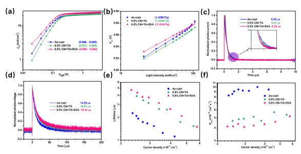
Fig. 5 (a) Photocurrent density ( $J_{ph}$ ) as a function of effective voltage ( $V_{eff}$ ) characteristics. (b) Light intensity dependence of  $V_{oc}$ . (c) Transient photocurrent and (d) transient photovoltage decay curves of the PTQ10:Y26 devices under different treatments. (e) Charge carrier lifetime *versus* charge density. (f) Bimolecular recombination rate constant  $K_{rec}$  *versus* different charge densities of PTQ10:Y26 devices.
