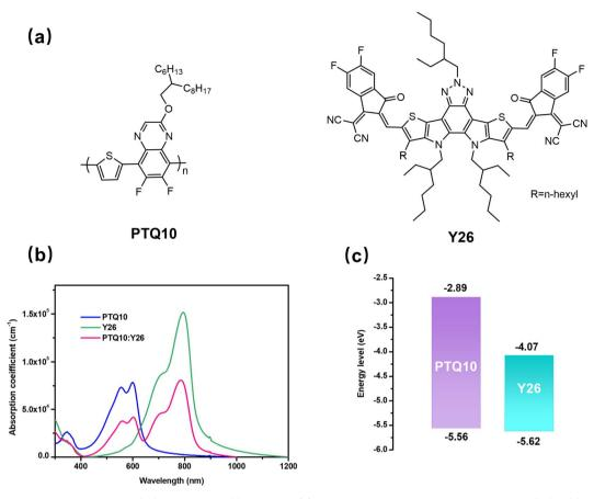
Fig. 1 (a) Chemical structures of the PTQ10 donor and Y26 acceptor. (b) UV-Vis-NIR absorption spectra of the PTQ10, Y26, and PTQ10:Y26 films. (c) Energy-level alignment of the donor PTQ10 and acceptor Y26.
