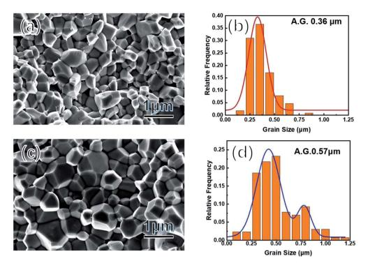
Fig. 3 (a and c) SEM images of freshly fractured surfaces of  $Co_{0.94}Ni_{0.06}SbS$  and  $Co_{0.94}Ni_{0.06}SbS_{0.96}Te_{0.04}$ , respectively; (b and d) their corresponding grain-size distribution analysis.
