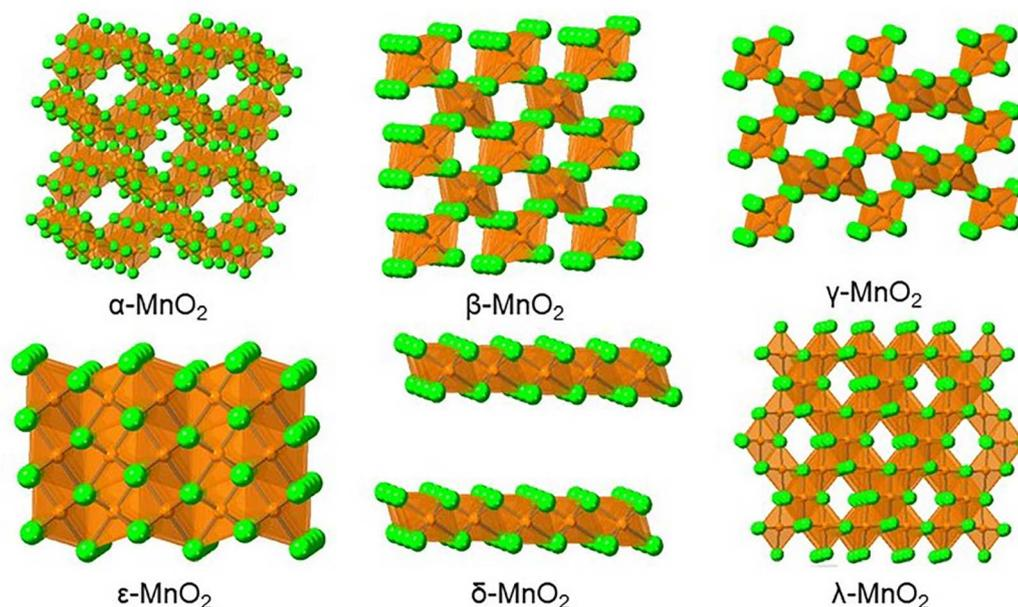
Fig. 3 Schematic diagram of the crystal structure of  $\alpha$ -,  $\beta$ -,  $\gamma$ -,  $\epsilon$ -,  $\delta$ - and  $\lambda$ -MnO<sub>2</sub>.
