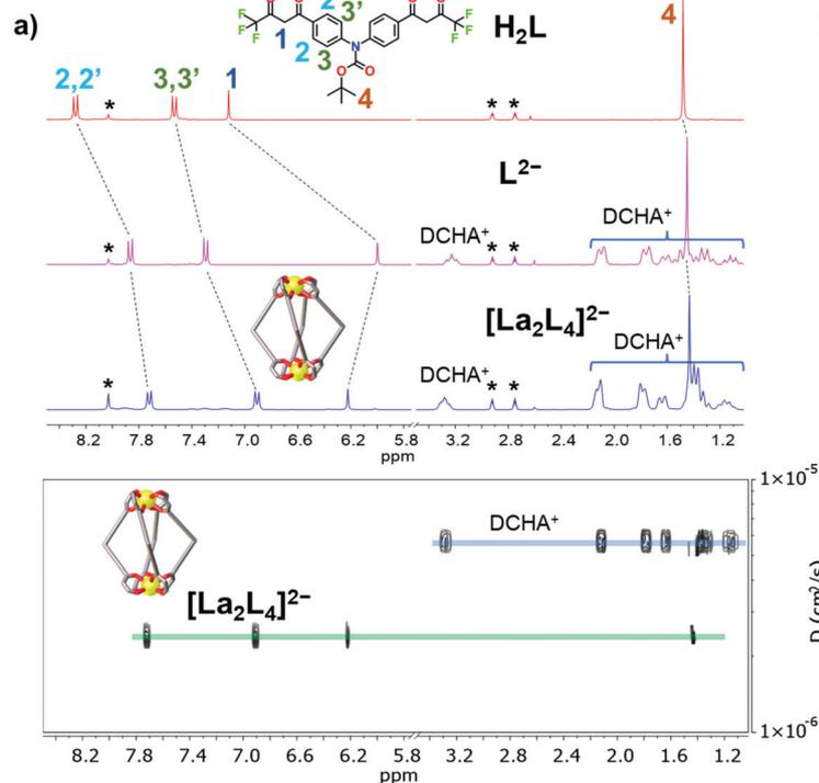
**Fig. 3** (a)  $^1H$ -NMR spectra (25 °C, 300 MHz,  $DMF-d_7$ ) of ligand  $H_2L$ , deprotonated ligand  $L^{2-}$  and the cage  $[La_2L_4]^{2-}$ . DOSY of  $[La_2L_4]^{2-}$ . \* =  $DMF$ . (b) Crystal structure of the Eu helicate,  $M$  and  $P$  forms in the asymmetric unit. H atoms and external  $NEt_4^+$  ions omitted for clarity. Color code: C, grey; O, red; N, blue; F, green; Eu, orange.
