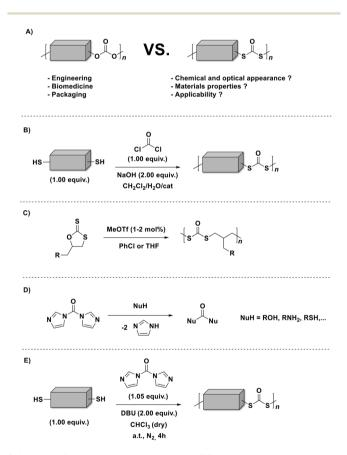
Scheme 1 Schematic representation of: (A) the replacement of oxygen with sulfur atoms in polycarbonates, resulting in polydithiocarbonates; previously reported approaches for polydithiocarbonate synthesis: (B) phosgene-based step-growth and (C) ring-opening polymerizations; (D) The reactivity of CDI with diverse nucleophiles; (E) the currently investigated CDI mediated polymerization for polydithiocarbonate synthesis in the presence of DBU.
