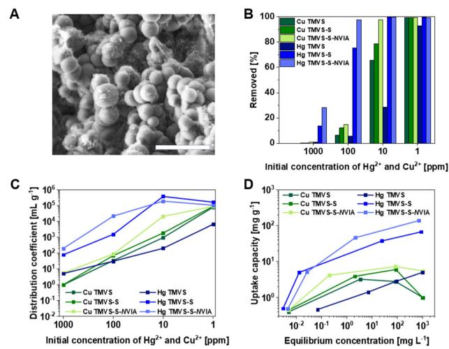
Fig. 2 (A) SEM image of TMVS-S-NVIA particles. Scalebar is 5 μm. (B) Removed copper ions (green) and mercury ions (blue) from aqueous solution by TMVS-S and TMVS-S-NVIA particles in %. Calculated distribution coefficients (C) and uptake capacities (D) of TMVS-S particles and TMVS-S-NVIA particles, respectively. Uptake capacities plotted against initial ion concentration can be found in the ESI.†
