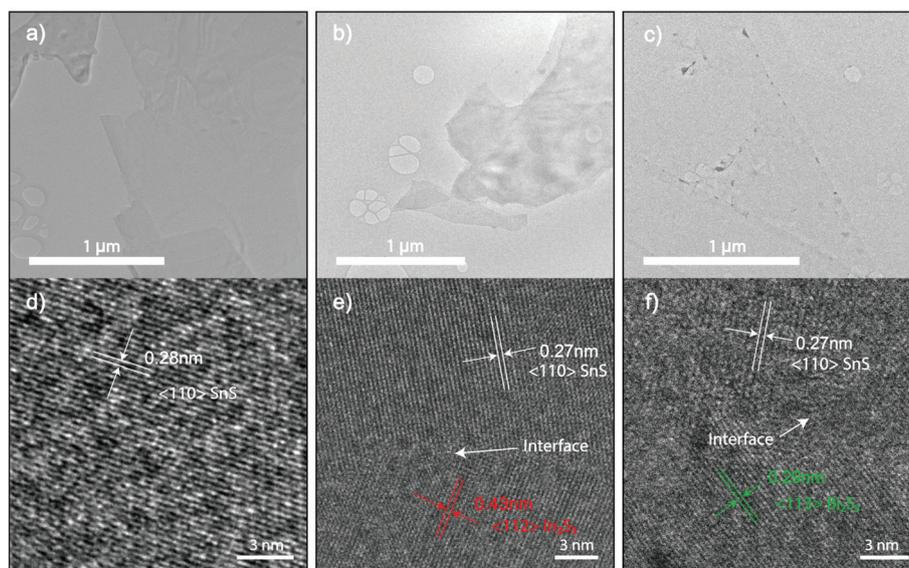
**Fig. 3** (a–c) The bright-field TEM image of undoped 2D SnS and 6.4 at% In and 0.1% Bi doped 2D SnS, respectively. (d–e) HRTEM images of the corresponding TEM images in a–c showing the formation of In<sub>2</sub>S<sub>3</sub> and Bi<sub>2</sub>S<sub>3</sub> grains. The sulphide doping formation is in agreement with the oxide counterpart.<sup>22</sup>
