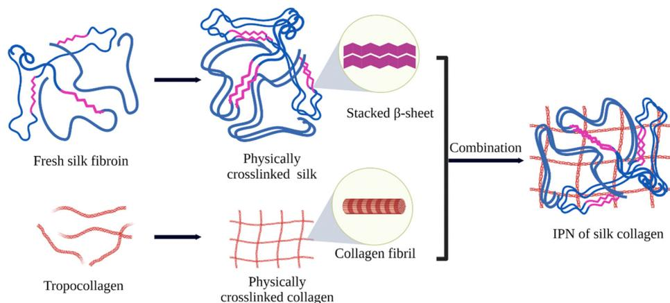
Fig. 12 Schematic illustration of the formation of physically crosslinked collagen–SF IPN. Reproduced with permission from Elsevier.<sup>156</sup>
