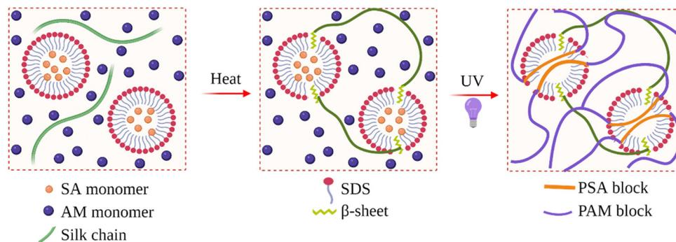
Fig. 14 Preparation of IPN hydrogels composed of SF and poly(acrylamide-co-stearyl acrylate). Reproduced with permission from Wiley-VCH, copyright 2019.<sup>163</sup>
