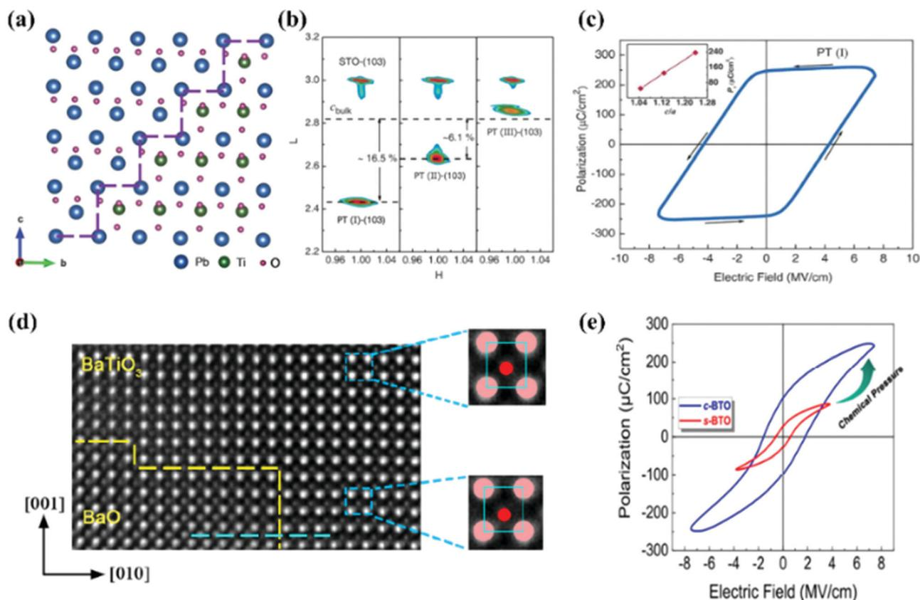
Fig. 3 (a) Crystallographic model of interphase strain between PTO and PbO; (b) Synchrotron X-ray reciprocal space mappings (RSMs) study of PT(I), PT(II), and PT(III) epitaxial thin films around the STO (103) plane, and (c)  $P$ - $E$  hysteresis loops of ultra-tetragonal PTO thin films;<sup>75</sup> The cross-sectional HAADF-STEM (d) and  $P$ - $E$  hysteresis loops (e) of c-BTO films.<sup>76</sup>
