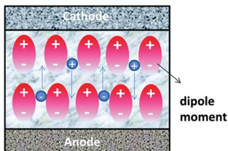
Fig. 9 The working principle of ferroelectric photovoltaic devices.<sup>149</sup>
