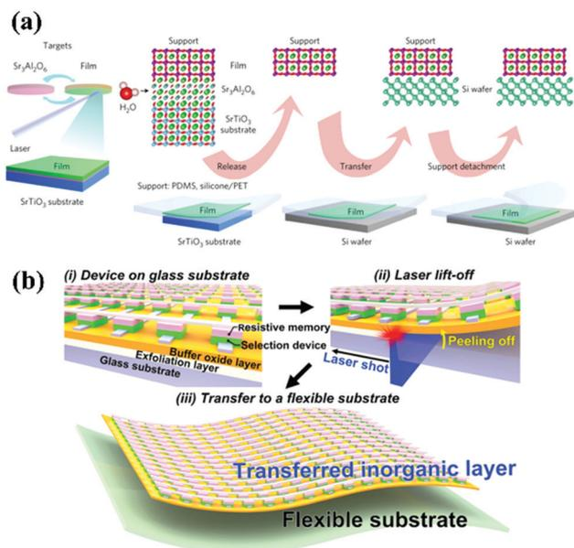
Fig. 10 (a) Process schematic of etching of the sacrificial layer to prepare flexible thin films.<sup>81</sup> (b) Schematic diagram of fabricating flexible thin films by a laser lift-off (LLO) process.<sup>191</sup>
