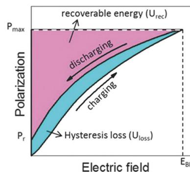
Fig. 8 The recoverable energy storage density and loss from  $P$ - $E$  loops of a dielectric capacitor.<sup>139</sup>
