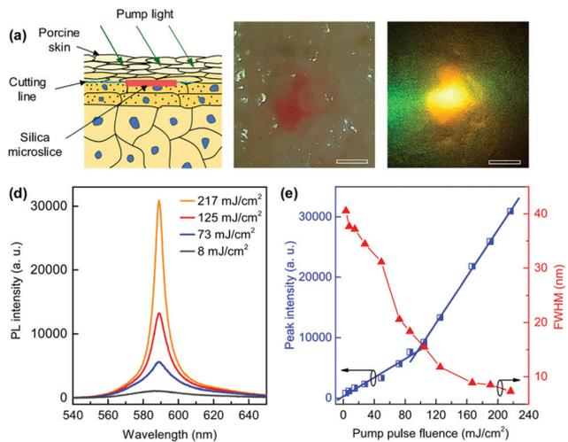
**Fig. 18** (a) Schematic of random lasers implanted into the skin. (b) Optical microscope image of a laser embedded below the porcine skin surface. (c) PL image of the sample upon optical excitation. (d) Emission spectra of the embedded laser sample at various pump fluences. (e) Peak intensity and FWHM of emission spectra versus pump fluence. (Reproduced from ref. 74, with permission from [Elsevier]).
