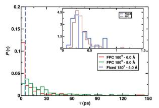
Fig. 4 Normalized reaction time distributions for CO + O recombination from 500 simulations, for reactions initiated from  $\theta$  = 180° and R = 4.0, 6.0,  $8.0~\mbox{\normalfont\AA}$  using fixed  $^{45,269}$  and fluctuating point charge (FPC) models. The inset reports the distribution for R = 4.0 Å and almost all recombination takes place within 1 ps. The reaction probability found with R = 4.0 Å is 32% and 99.2% with fixed and fluctuating charges respectively.
