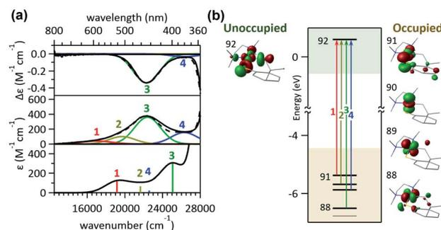
Fig. 4 (a) 5 T MCD (top), Abs (middle), and TDDFT-simulated Abs (bottom) spectra of **1**<sub>tmeda</sub>. The deconvoluted Gaussian bands and their sum spectra are shown in colored solid and black dashed lines, respectively. (b) MO diagram of **1**<sub>tmeda</sub> and frontier MOs relevant to the electronic transitions in the visible region.
