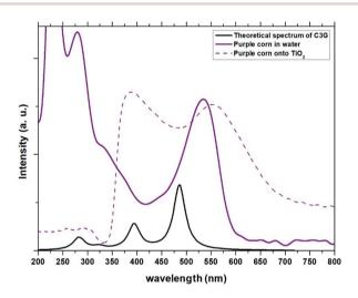
Fig. 3 Experimental absorption spectra of the dye obtained from *Zea mays* in solution and adhered to TiO<sub>2</sub> compared with the theoretical spectrum obtained for C3G.
