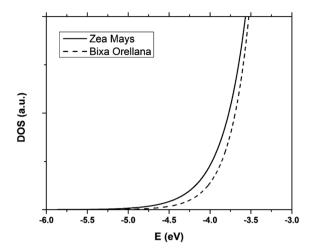
Fig. 10 Distribution of the density of trap states of TiO<sub>2</sub> in cells manufactured with Zea mays and Bixa orellana.
