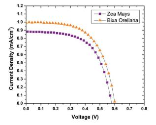
Fig. 5 Current–voltage curves of the devices manufactured with Zea mays and Bixa orellana.
