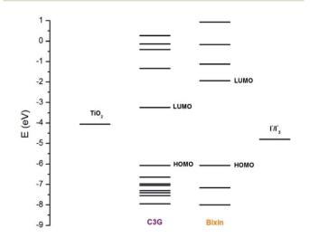
Fig. 1 Energy levels of the molecular orbitals of C3G and bixin. The energy levels of the redox couple  $I^-/I^{3-}$  (-4.9 eV) and of the conduction bank of TiO<sub>2</sub> (-4.0 eV) are also shown in the diagram.
