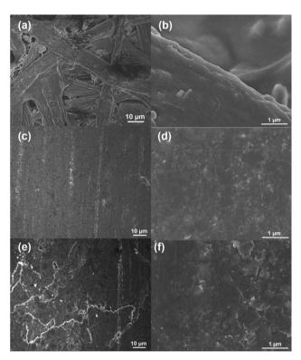
Fig. 2 SEM images with different magnifications of  $1000\times$  and  $20\ 000\times$ : (a and b) office paper, (c and d) non-treated PDEs, and (e and f) CO<sub>2</sub> laser-treated PDEs.
