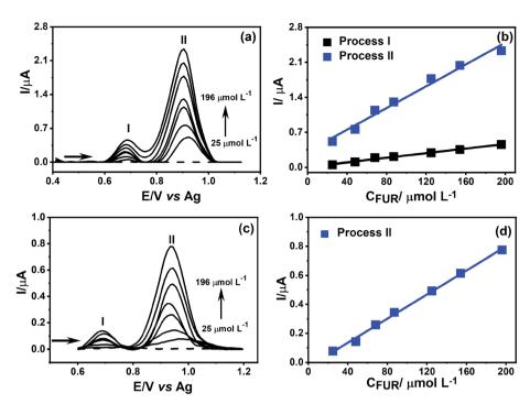
Fig. 7 DPVs recorded using (a)  $CO_2$  laser-treated and (c)  $CO_2$  non-treated PDEs in 0.1 mol  $L^{-1}$  PBS (pH = 6.8) (dashed lines) containing 25, 48, 68, 87, 125, 154, and 196  $\mu$ mol  $L^{-1}$  FUR (solid lines), (b and d) calibration curves obtained from FUR measurements for both  $CO_2$  laser-treated and non-treated PDEs, respectively. Parameters: scan rate: 20 mV s<sup>-1</sup>, amplitude: 50 mV, and step: 10 mV.
