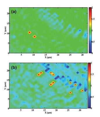
Fig. 3 Raman mappings showing  $I_{\rm D}/I_{\rm G}$  ratio of (a) non-treated and (b) CO<sub>2</sub> laser-treated PDEs.
