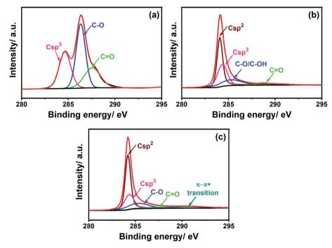
Fig. 4 High-resolution C 1s XPS spectra of (a) office paper, (b) non-treated PDEs, and (c) CO<sub>2</sub> laser-treated PDEs.
