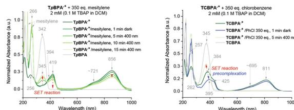
**Fig. 9** UV-vis spectra of **TpBPA<sup>+</sup>** (top) and **TCBPA<sup>+</sup>** (bottom) in the presence of mesitylene and PhCl, respectively and after irradiation at 395 nm.
