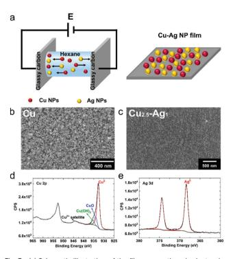
Fig. 3 (a) Schematic illustration of the film preparation via electrophoresis. The arrows indicate the moving direction of NPs under applied potential. (b and c) SEM images of the anode Cu (b) and Cu<sub>2.5</sub>-Ag<sub>1</sub> (c) NPs film prepared at 100 V for 60 min. (d and e) Cu 2p (d) and Ag 3d (e) XPS spectra of a Cu<sub>2.5</sub>-Ag<sub>1</sub> NPs film prepared by electrophoresis at 100 V for 60 min.
