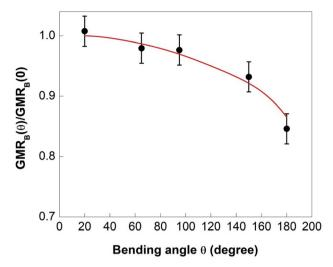
Fig. 7 Experimental GMR<sub>B</sub>( $\theta$ ) ratio (dots) normalized to the value measured on the flat sample ( $\theta=0^{\circ}$ ). Calculated values using eqn (1) are marked by a red line.
