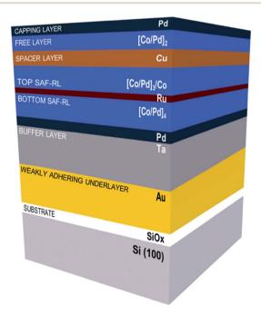
Fig. 1 Schematic sample structure of the Co/Pd-based GMR-SV stack consisting of a [Co/Pd]<sub>4</sub>/Ru/[Co/Pd]<sub>3</sub>/Co synthetic antiferromagnet reference layer (SAF-RL) and a [Co/Pd]<sub>2</sub> free layer separated by a Cu spacer layer. Reference samples were directly deposited on SiO<sub>x</sub>/ Si(100) substrates, while a weakly adhering Au underlayer was interposed to allow for the transfer of the stack on a flexible tape.
