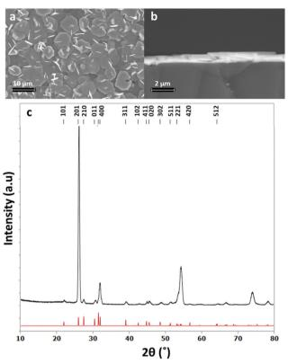
Fig. 4 Top down SEM image (a), cross sectional SEM image (b) and grazing incidence XRD pattern (c) for SnS thin film obtained by low pressure CVD using  $[Sn^nBu(S^nBu)_2]$  (red = XRD pattern for bulk  $SnS^{48}$ ) with a thickness of around 700 nm.
