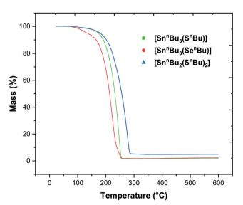
Fig. 1 TGA profiles for (1) (green), (2) (blue) and (3) (red). The TGA experiments were conducted with a temperature ramp rate of 5  $^{\circ}$ C min $^{-1}$  and a constant flow of argon gas at a flow rate of 30 mL min $^{-1}$ .
