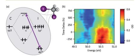
Fig. 9 (a) Term scheme of the diiodomethane  $(CH_2I_2)$  target molecule. The resonant XUV excitation from the iodine 4d orbital to an antibonding  $\sigma^*$  molecular orbital is indicated by the violet arrow. (b) XUV-pump XUV-probe transient absorption spectroscopy of diiodomethane (probe-pulse spectrum).
