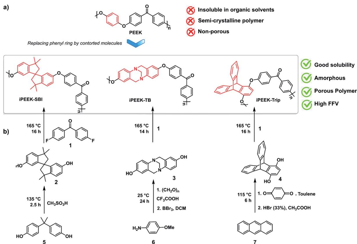
**Scheme 1** (a) The concept of molecular fusion of PEEK and PIM into intrinsically microporous poly(ether-ether-ketone) (iPEEK) by the substitution of the phenyl ring in PEEK by contorted structures to enhance the fractional free volume (FFV), porosity and the solution-processability. (b) Synthetic route for the contorted, diol monomers and their corresponding polymers.
