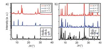
Fig. 2 Structural properties of thin films. XRD patterns of (a) A2- $FA_{n-1}Pb_nI_{3n+1}$  and (b)  $A'_2FA_{n-1}Pb_nI_{3n+1}$  on FTO/mp-TiO<sub>2</sub> substrates for n=1 (black), n=2 (blue) and n=3 (red) compositions in accordance with the previous report.<sup>13</sup> Inset shows DFT-optimised (B3LYP/6-31G(d)) structures of the spacers (a) A and (b) A'.
