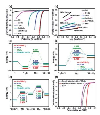
Fig. 3 (a) HER polarization curves of porous CoP/MoO $_2$ , CoP, CoMoO $_4$ , MoO $_2$ , pure CC and commercial Pt/C (20%) in 1 M KOH solution. (b) The Tafel plots corresponding to a. (c–e) Calculated transition state adsorption energy diagram of the HER for CoMoO $_4$ , CoP, MoO $_2$  and CoP/MoO $_2$ , in which TS1, TS2, TS3 and TS4 represent the energy barriers for the reaction. (f) Comparison of polarization curves for porous CoP/MoO $_2$ , non-porous CoP/MoO $_2$  and pure CoP thin films.
