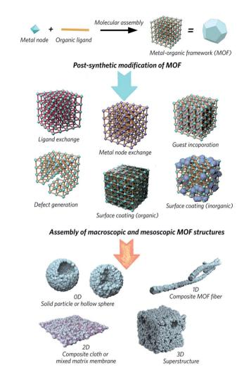
Fig. 1 Schematic overview of post-synthetic modifications and meso/ macroscopic morphological assemblies of MOFs.
