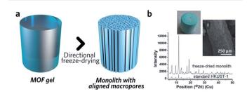
Fig. 8 Freeze drying to introduce aligned macropores to monolithic MOF. (a) Schematic diagram of the freeze-drying process. (b) PXRD, optical photo and SEM image of the HKUST-1 monolith with aligned macropores. Reproduced from ref. 89 with permission from the Royal Society of Chemistry, copyright 2015.
