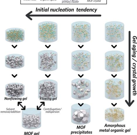
Fig. 2 Mechanism of the formation of a MOF gel, precipitate and metal—organic gel.
