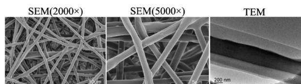
Fig. 5 SEM and TEM images of double drug-loaded nanofibers with core-sheath structure.<sup>102</sup> Copyright 2018, Elsevier.
