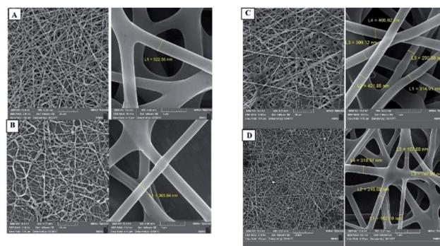
Fig. 8 Effects of different parameters (voltage, flow velocity) on the fiber diameter.<sup>133</sup> Copyright 2018, Elsevier. (A) 20 kV, 0.5 ml h<sup>-1</sup>; (B) 20 kV, 0.1 ml h<sup>-1</sup>; (C) 30 kV, 0.5 ml h<sup>-1</sup>; (D) 30 kV, 0.1 ml h<sup>-1</sup>.
