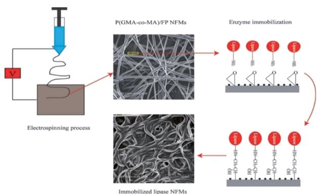
Fig. 7 Schematic diagram of the preparation process of lipase immobilized on electrospun nanofibers.<sup>131</sup> Copyright 2018, Elsevier.
