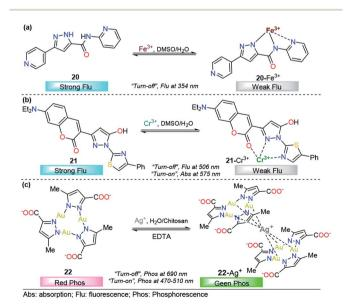
Fig. 12 Probes for Fe<sup>3+</sup>, Cr<sup>3+</sup> and Ag<sup>+</sup> based on pyrazoles (a) 20, (b) 21 and (c) 22.
