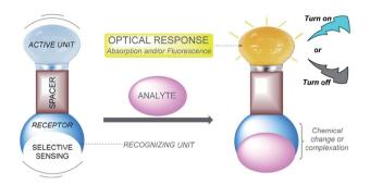
Fig. 1 Schematic representation of a colorimetric/fluorescent chemosensor.
