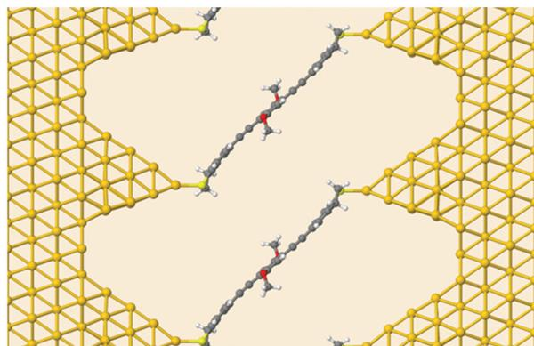
Fig. 6 Device geometry for DFTB transport simulations. Shown is OPE3-Ph(OMe)<sub>2</sub> connected to semi-infinite gold leads.
