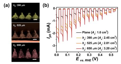
Fig. 4 (a) Optical images of the fabricated 3D photoelectrodes composed of 400 pyramids. The total light absorption area ( $A_a$ ) of the 3D photoelectrodes is modulated by adjusting  $h_p$  to 390, 525, and 650  $\mu$ m (fixed  $L_b$ : 490  $\mu$ m). The scale bar is 250  $\mu$ m. (b) Chopped-light PEC performance of the p-n homojunction Cu<sub>2</sub>O electrodes with planar and 3D pyramid shapes with respect to the total light absorption area ( $A_a$ ).
