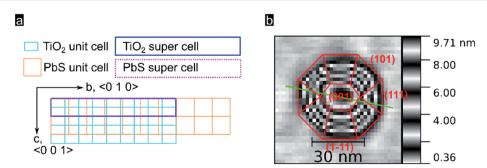
Fig. 3 (a) Lattice of  $TiO_2$  rutile (100) surface, turquoise, superimposed by a lattice of PbS (100), orange. Calculated matching supercells are marked with a blue rectangle for the  $TiO_2$  supercell and a dotted purple rectangle for the PbS supercell. (b) Representation of a quantum dot with crystal facets inferred following Moll *et al.*<sup>53</sup>
