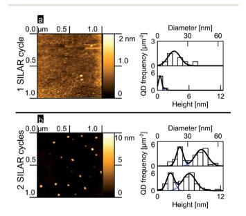
Fig. 1 PbS SILAR on rutile (100) (a) 1 cycle, AFM image, QD height and diameter histograms and fits (b) likewise, but for 2 cycles.
