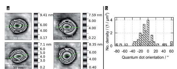
Fig. 2 (a) Selected AFM images of PbS QDs on (100) rutile TiO<sub>2</sub>; green lines are the estimated orientation of their long QD axis as described in the body text (b) histogram showing the preferential orientation for the QDs nucleated by SILARs.
