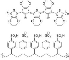
Fig. 1 Structure of PEDOT:PSS.
