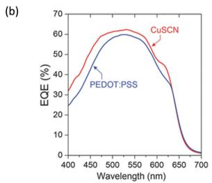
Fig. 9 (a) Transmittance of CuSCN compared to PEDOT:PSS (top), and (b) EQE plots for P3HT:ICBA-based OPV devices containing the two hole transport layers.<sup>72</sup> Reproduced with permission.<sup>72</sup> Copyright 2015, WILEY-VCH Verlag GmbH & Co. KGaA, Weinheim.
