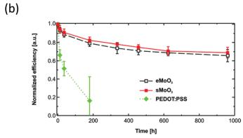
Fig. 8 (a) X-Ray photoelectron spectroscopy of solution-processed  $MoO_3$  (s $MoO_3$ ) compared to an evaporated film (e $MoO_3$ ) and (b) stability of OPV devices with P3HT:PC<sub>61</sub>BM active layer, stored in ambient conditions reported by Rand *et al.*<sup>60</sup> Reprinted with permission from ref. 60. Copyright 2011 American Chemical Society.
